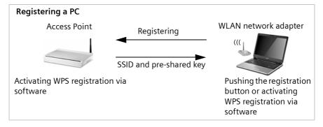
The first time this button is pressed, the device automatically creates a SSID and a pre-shared key, if these had not been already set on delivery or has been configured before manually. If a client activates WPS registration within the two-minute interval, the security data is exchanged and a connection is established. Only **one** client may synchronise during the two-minute interval. After the successful synchronization the registration is closed.
