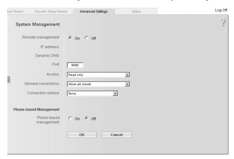
Remote Management enables a PC that is not in your local network to be used to configure the Gigaset SX763 WLAN dsl via a standard Web browser. You can activate Remote Management for one particular or for any PC.
