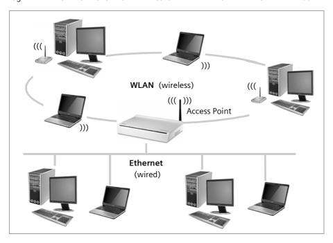
The Gigaset SX763 WLAN dsl has four Ethernet interfaces (LAN ports). Up to four PCs can be connected directly to these LAN ports.
