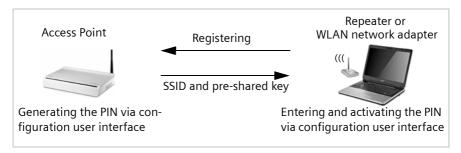
WLAN adapters without WPS can also be set up manually, i.e. the SSID and key must be entered manually. How you can find out which SSID and which pre-shared key is set, you can read in chapter "Configuring wireless connections" on page 85.
