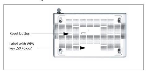
**Reboot function**: Press and hold the right end of the button for more than 1 second but less than 5 seconds to reboot the device. This does not affect the configuration settings.
