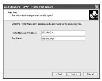
→ In the *Printer Name or IP Address* input field, enter the IP address of the print server (Gigaset SX763 WLAN dsl): e.g. 192.168.2.1.
