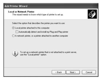
The printer port you are installing will behave like an additional parallel port on the PC. For this reason you must click the option button next to *Local printer* in this window.
