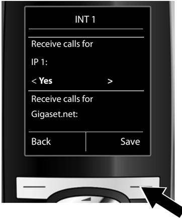
If no calls to the VoIP connection **IP 1** are to be signalled on the handset:
