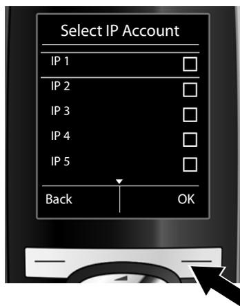
A list of all possible IP connections is shown in the display (IP 1 to IP 6). VoIP connections that are already configured are marked with .
