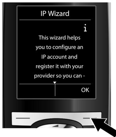
> Press the bottom of the control key
