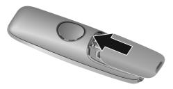
▶ Slide the battery cover back into the main casing until it clicks into place.
