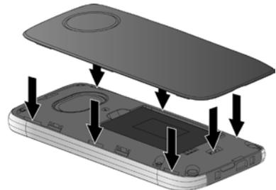
To **reopen the battery cover** to replace the battery:
