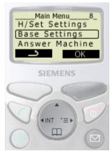
2. Select "Base Settings", press control key and confirm with display key ok.
