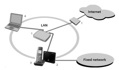
Figure 1 Connecting the phone to the fixed network and the Internet
