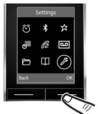
Use the right, left, down, and up Control key to navigate to the Settings submenu.
