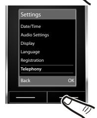
▶ Press down on the Control key until the **Telephony** menu appears on the display.
