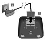
Connect the flat plug from the power supply 1.
