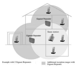
Before you start to register the units, install the Gigaset Repeater in close proximity to the base station and a power supply point. If a Gigaset Repeater is already in use, it must be switched on and positioned next to the base station before registration can commence.
