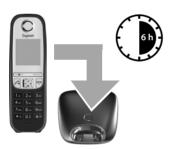
Charge the handset in the base station/charging cradle for 6 hours.
