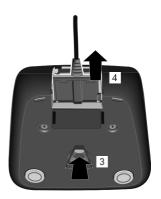
If you need to disconnect the plug from the charging cradle, press the release button 3 and disconnect the plug 4.
