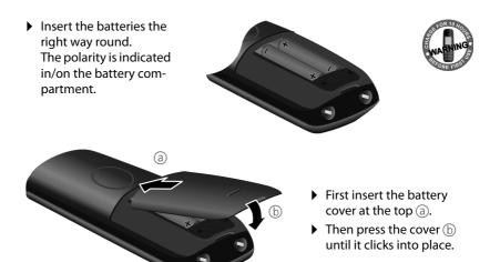
If you need to open the battery cover, for instance to replace the batteries, place your fingertip in the cavity on the casing and pull the battery cover upwards.
