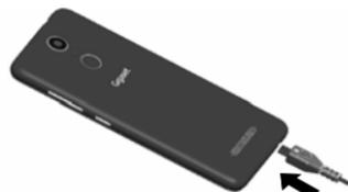
The Message LED lights red during the charging process (→ p. 3). The device is charged once the Message LED lights green and the charge icon
