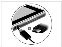
Insert the small end of the USB cable into the micro USB port of the device horizontally, without tilting it ■1.
